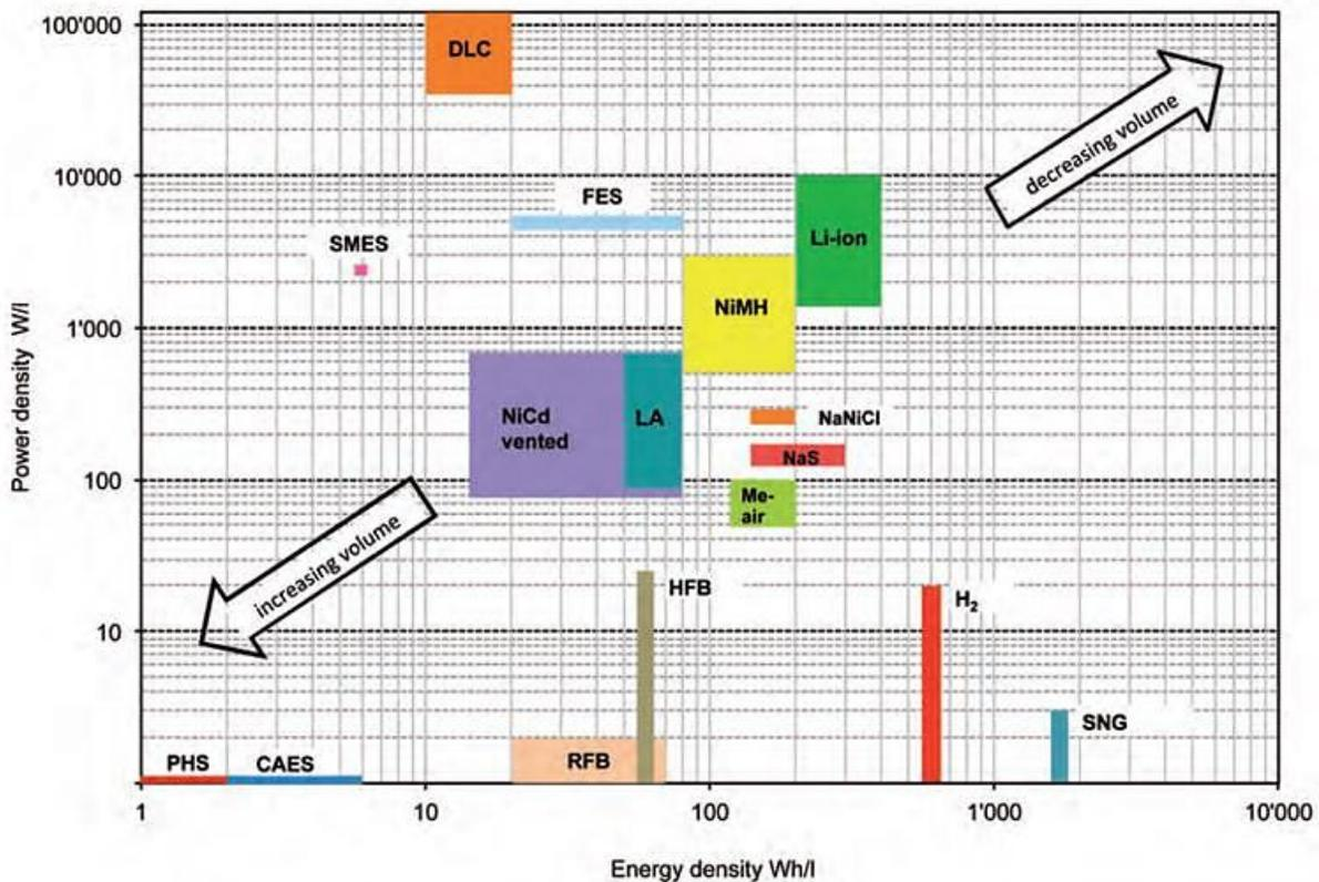
Figure 2.10. Comparison of power density and energy density (in relation to volume) of energy storage technologies
