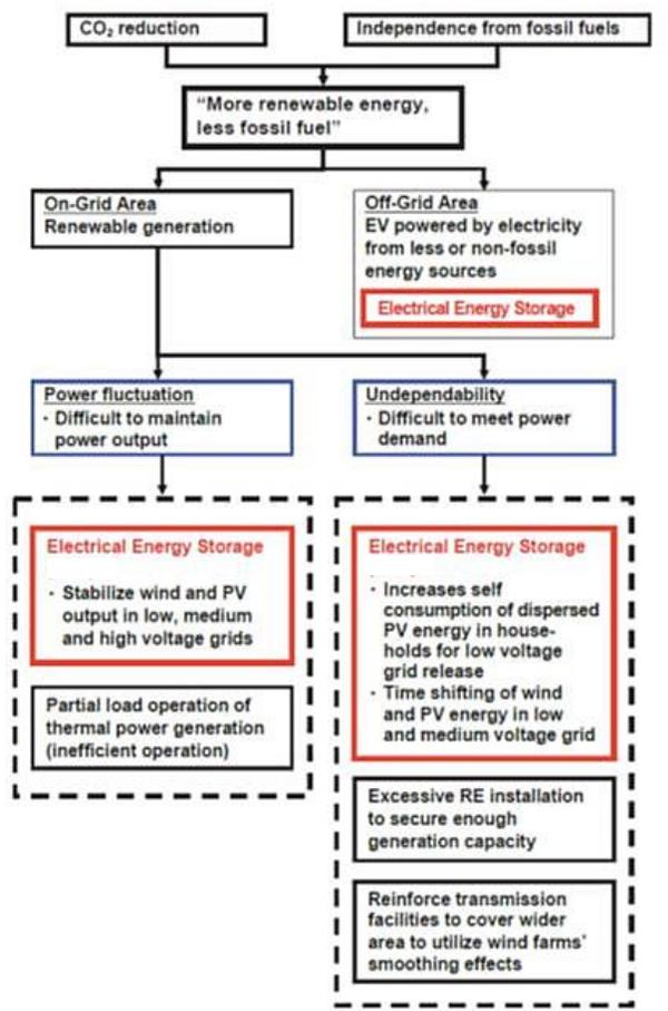
Figure 1.2. Problems in renewable energy installation and possible solutions. (RE: Renewable energies)
