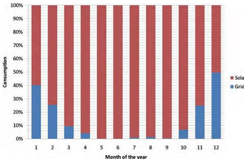
Figure 3.8. Consumption of a typical household with a storage system: energy consumed from the grid and from the photovoltaic system.
