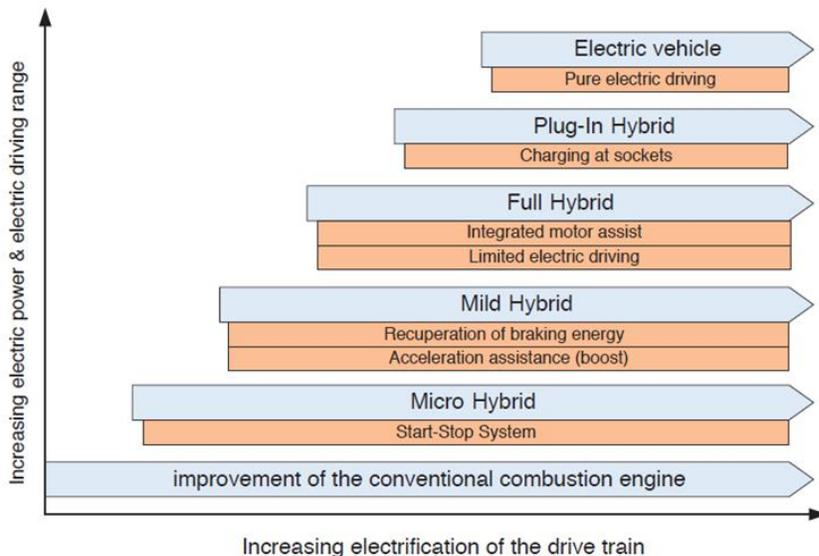
Figure 3.16. Hybrid classes sorted by electrical power and functional range, against stage of development
