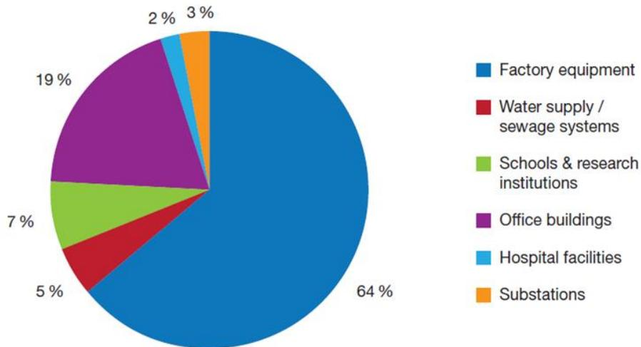
Figure 3.5. Locations of NaS systems in service area
