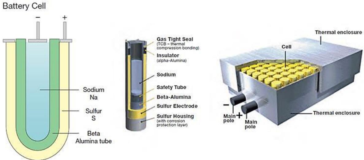
Figure 2.6. NAS Battery cell design and 50 kW module (NGK)
