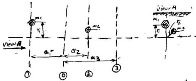
Figure 5. An example to balance a shaft dynamically.
