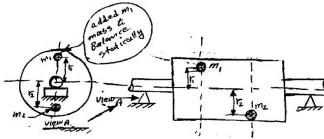
Figure 3. Static balancing of a rotating shaft.
