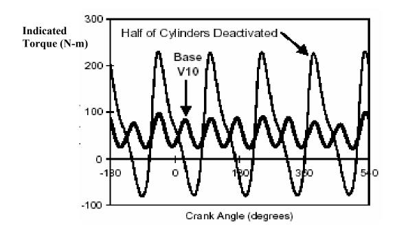
Figure 1. Torque pulsation as a function of crank angle showing the base engine (10-cylinder) and when half of the cylinders were deactivated. 500 rpm at 0.8 bar BMEP.
