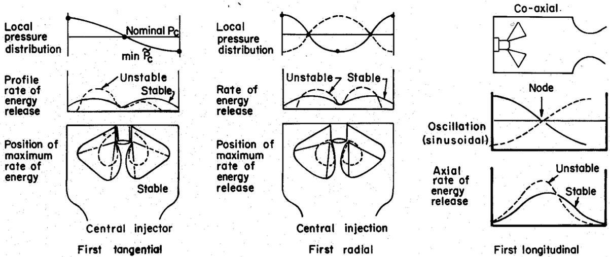
Schematic comparison of resonant combustion and steady-state energy release patterns for central injection.
