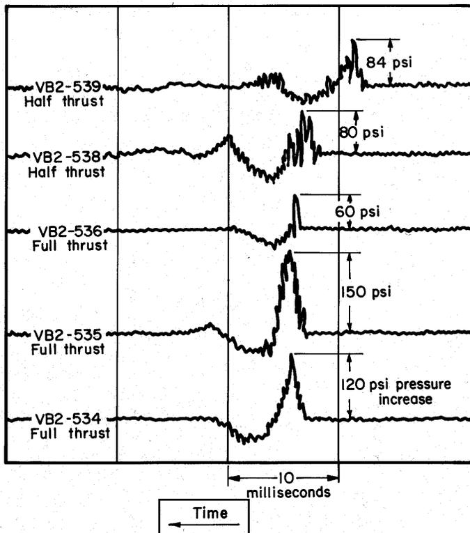
Typical pressure recovery for central injection design in LMDE engine.
