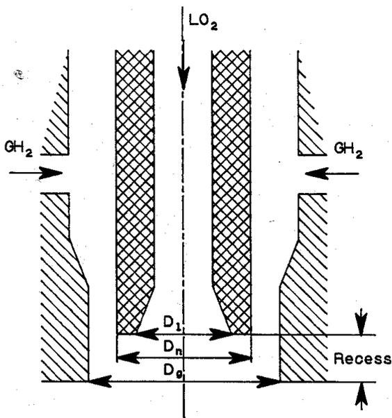
Typical coaxial injector
