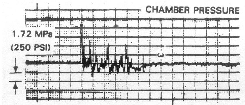
**Pressure trace exhibiting damping characteristics of FRT injector of F-1 engine**
