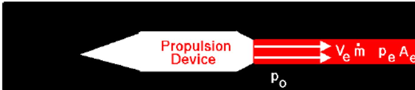
**Rocket Thrust Equation**  $F = \dot{m} V_e + (p_e - p_o) A_e$
